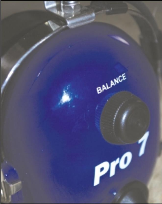
Photo E. The balance control helps ease fatigue during contests.
