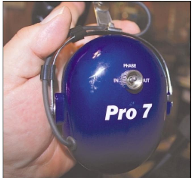
Photo F. The phase control makes a big difference in digging out the weak ones.
