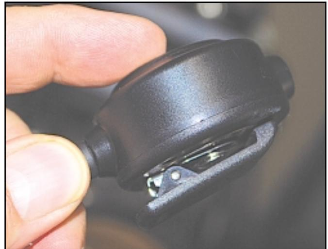
Photo G. Pictured is the Pro 7's PTT (push-to-talk) switch that can either rest on a desk or be clipped to a belt.
